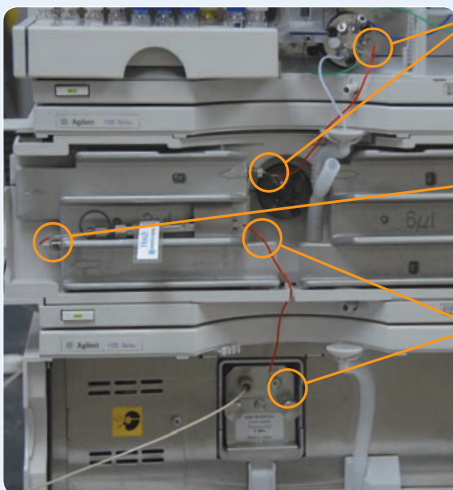
FIGURE 4: Replace standard capillary tubing (0.17 mm, green) with low volume capillary tubing (0.12 mm, red).
