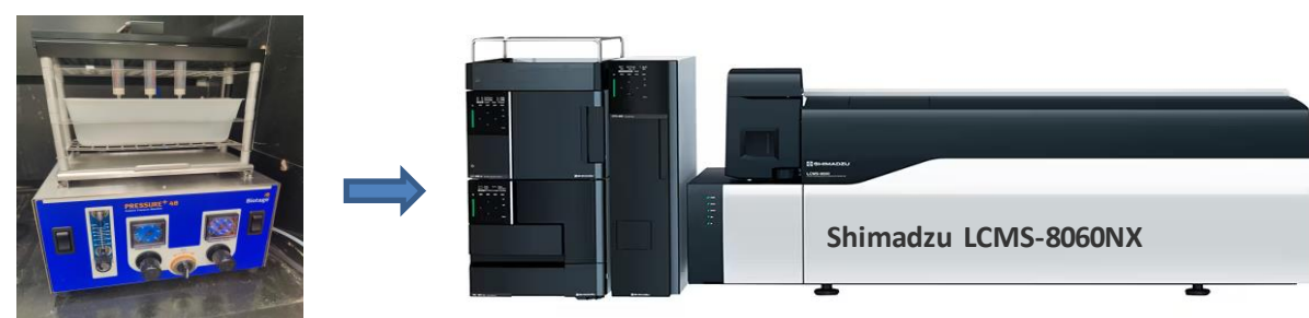
Fig. 2. Experimental workflow: Solid phase extraction → LC-MS/MS
