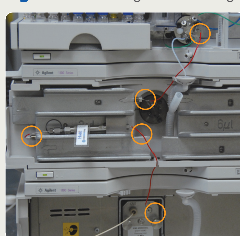
Figure 4: Reducing ECV in an Agilent 1100
